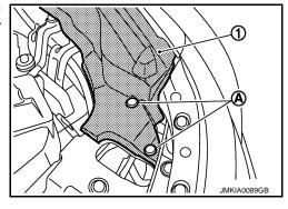
Remove bolts (A) of fixing bumper fascia and front fender (LH/ RH), using a tool (B).
