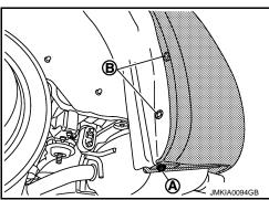
Remove screws (A) of bumper fascia front end upper (LH/RH).
