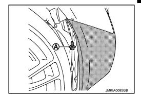
7. Remove clips of bumper fascia underside, and then pull out bumper fascia toward rear of vehicle.
