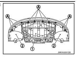
7. Remove fender protector (front) mounting bolts and clips, and then remove screws (A) of fixing bumper fascia left and right side.
