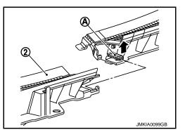
8. Plastic pawl (B) is push down and cowl top cover LH (1) is removed ahead of vehicles.
