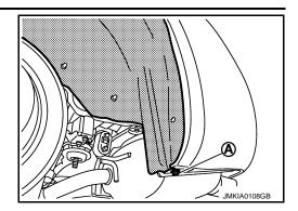
2. Remove screws (A) of rear wheel house protector located center mud guard.
